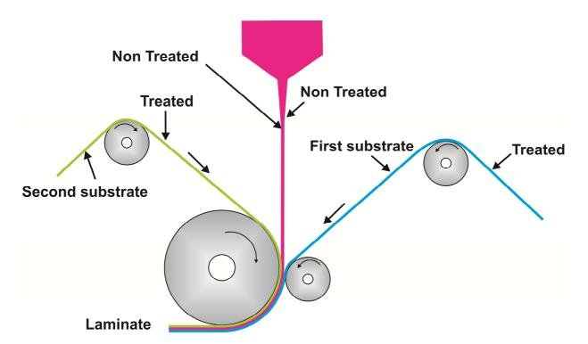
As it is clear in the above diagram that during Extrusion Coating we can do Corona Treatment on the first and second substrate but we cannot do Corona Treatment on the Hot Melt Poly.
