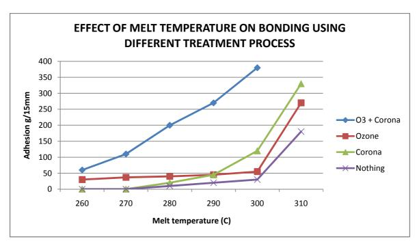
The research and experiments also show that if the ozone is applied near the nip at a distance of 4 cm from the hot melt poly. The adhesion achieved is maximum.
