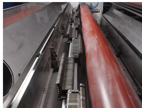
Fig 9: Aluminium/Steel - Fixed/ Segmented Width Electrodes
