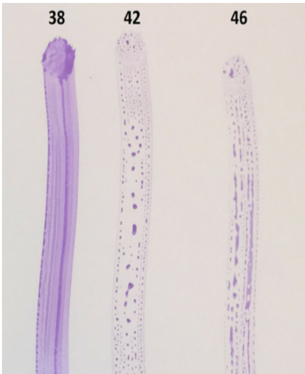
Fig. 34 No droplets were formed using number 38 dyne pen. Small amount of droplets can be seen with number 42 dyne pen. Complete droplets were formed within 2 seconds using number 46 dyne pen. Thus, dyne level of the substrate is 38-41.
